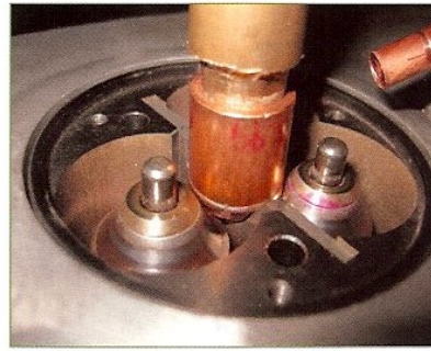
Fig. 10 — The hybrid dresser reforms the side by a roller and mills only the electrode's face.
