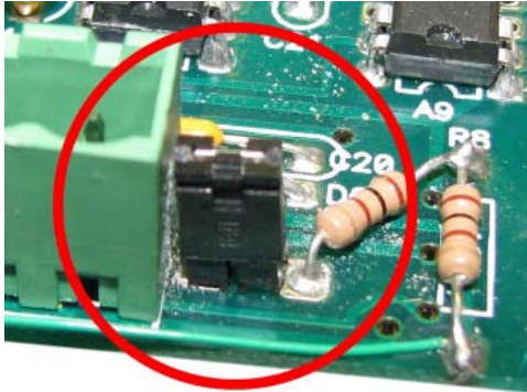
Figure 7-10. Sinking Sensor Jumper detail
