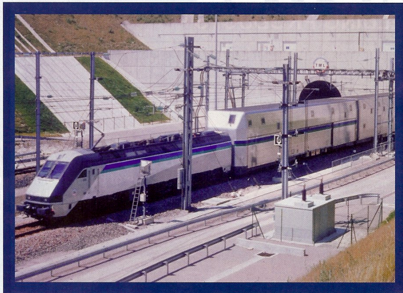
Bombardier Transportation's facility in La Pocatière, Québec, Canada, produced carshells of the Eurotunnel shuttle cars, the largest stainless steel cars ever made. The locomotive is of the standard size. (Photo courtesy of the Nickel Institute.)
