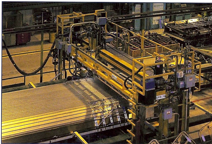
Fig. 8 — Specialized gantry machines with separate but synchronized mechanical systems for top and bottom electrodes are the solution for welding roof and side skin to their structures. (Photo courtesy of Bombardier.)
