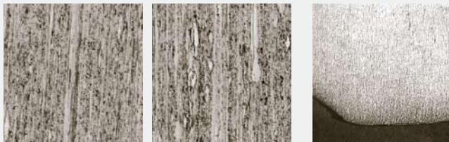
Nitrode before and after annealing at 900°
