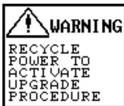
If pressed by accident, simply switch off the instrument, switch it back on again (nothing shows on the display), switch off and switch back on again.
