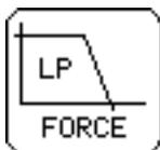
FORCE FILTER - For activating a filter on the disturbances present on the force measurement, which can occur in the presence of an electrical axis.
