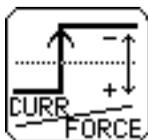
TRIGGER TYPE - The instrument normally receives the welding process start signal on both the current and the voltage channel; one of the two channels may be excluded from receiving the welding process start signal.
