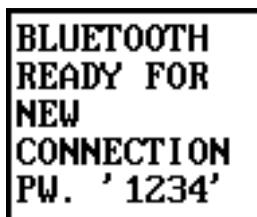
The instrument can now be detected by an external device.
