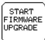
Pressing this key sets the instrument to firmware upgrade mode and the following message appears.
