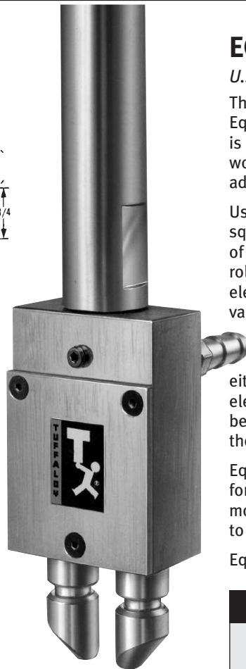
5 RW taper adapter shank, Part No. 195-5680
