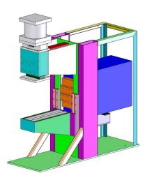
The main frame is high quality welded steel construction styled for trim appearance and functional design. The slim design requires a minimum of floor space. The upper arm extension is built integrally with the frame. The removable rear cover permits ready access to the frame interior for inspection and maintenance.
