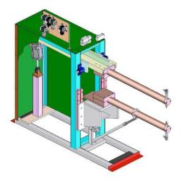
The main frame is high quality welded steel construction styled for trim appearance and functional design. The slim design requires a minimum of floor space. The upper arm extension is built integrally with the frame. The removable rear cover permits ready access to the frame interior for inspection and maintenance.
