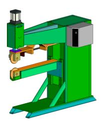
The main frame is high quality welded steel construction styled for trim appearance and functional design. The slim design requires a minimum of floor space. The upper arm extension is built integrally with the frame. The lower knee is steel, and supports the transformer; this allows the transformer to move up and down with the lower knee. A removable rear cover permits ready access to the frame interior for inspection and maintenance.
